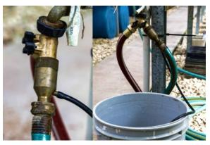
1. An eductor is a simple and cost effective way of applying chemical and fertilizer drenches, just double check the system to be sure it is mixing at the intended rate.
