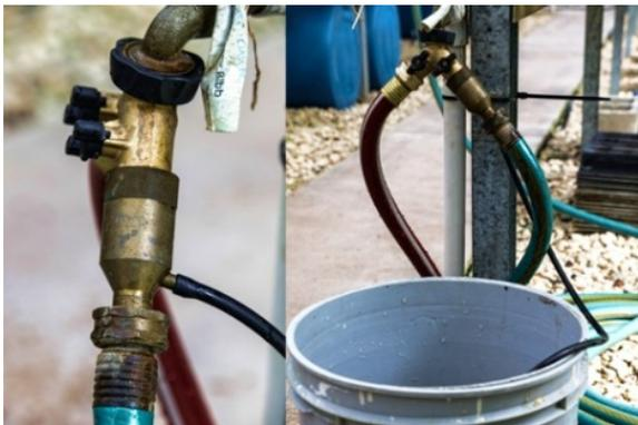
*Siphon.* For hobbyists with the need to mix up more than a few jugs of a drench solution, a siphonex may be the answer. A siphonex is a venturi device normally installed on the hose bib with the flexible suction hose dropped in a concentrated solution that is drawn into the hose by differential pressure. The [Hozon](#) operates at a 16:1 ratio and the [Dramm siphonject](#) has a 20:1 ratio, both cost less than \$30.
