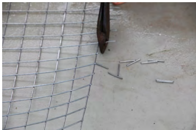
6. Remove the extra wire using snips to prevent blood loss later. That protruding wire catches on everything.
