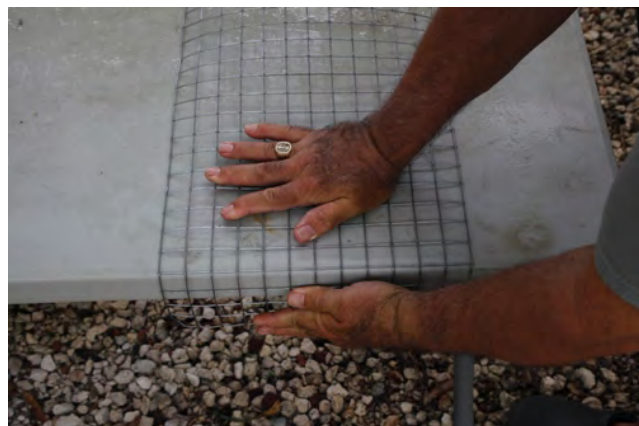
7. Bend each end of the basket, wires will be attached later.
